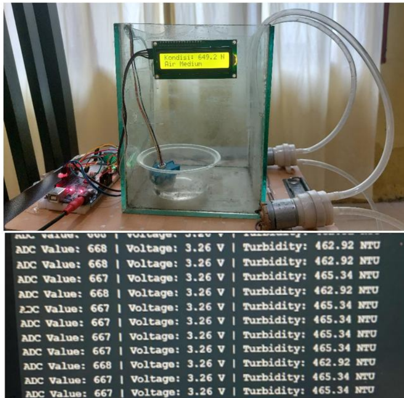
Gambar 2. Proses Pengujian Sensor Turbidity
